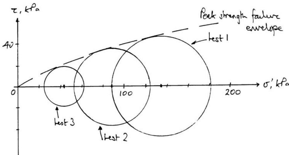
Figure Q5.2a: Mohr circles of stress at peak stress ratios  $(t/s')_{peak}$
