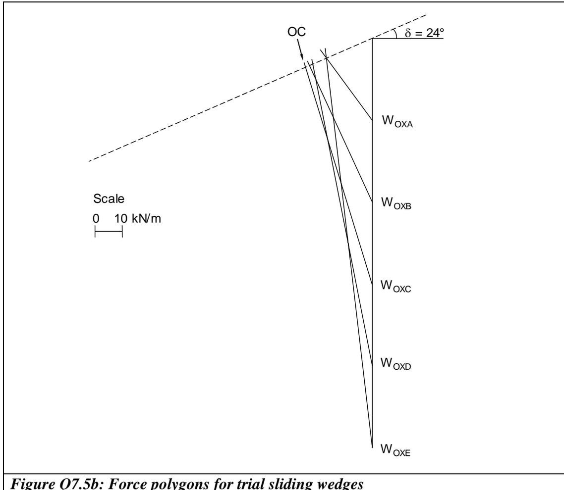
**Figure Q7.5b: Force polygons for trial sliding wedges**
