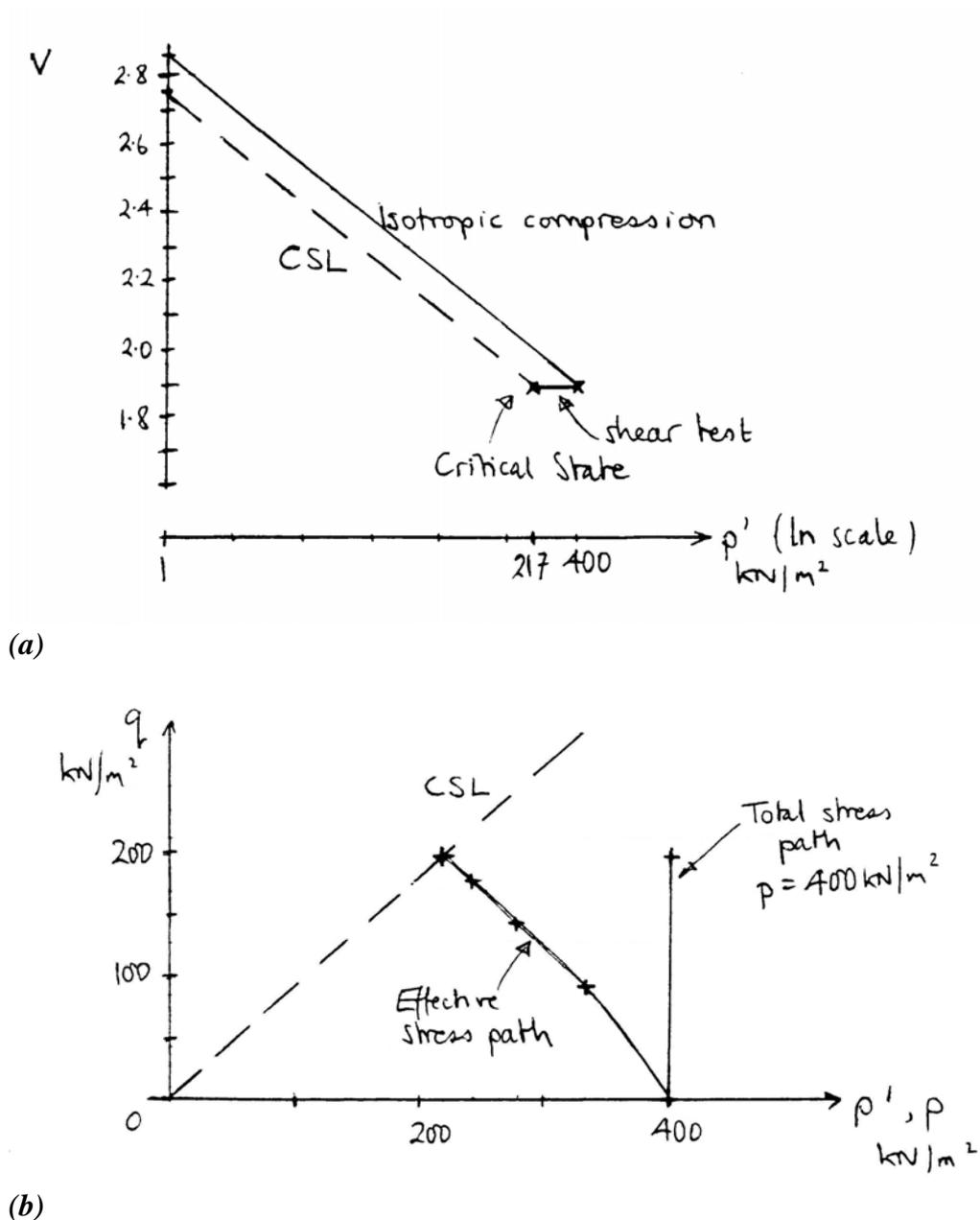
**Figure Q5.8:** (a)  $v$  against  $\ln p'$ ; (b)  $q$  against  $p$  and  $p'$
