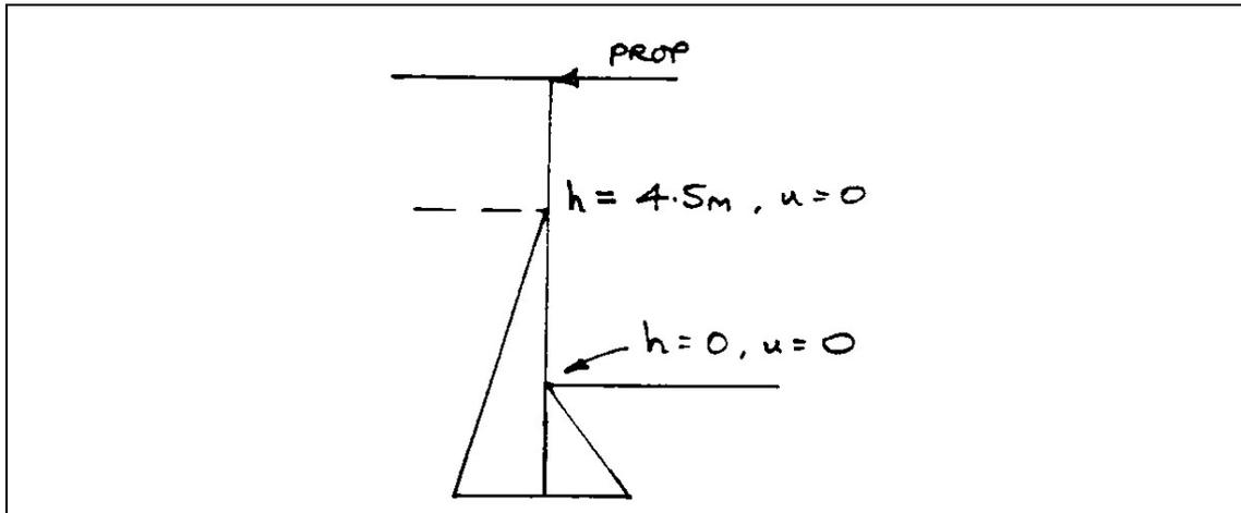
**Figure Q7.3a: Pore water pressures according to the linear seepage approximation**
