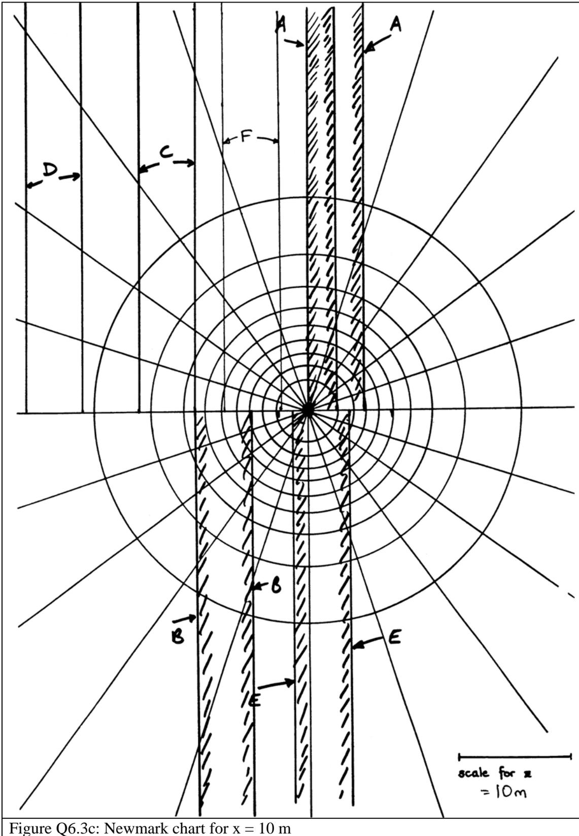
Figure Q6.3c: Newmark chart for  $x = 10$  m
