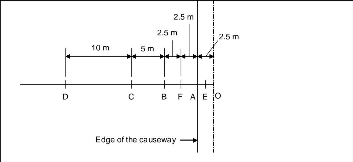
Figure Q6.3a: location of settlement calculation points relative to the centreline of the causeway
