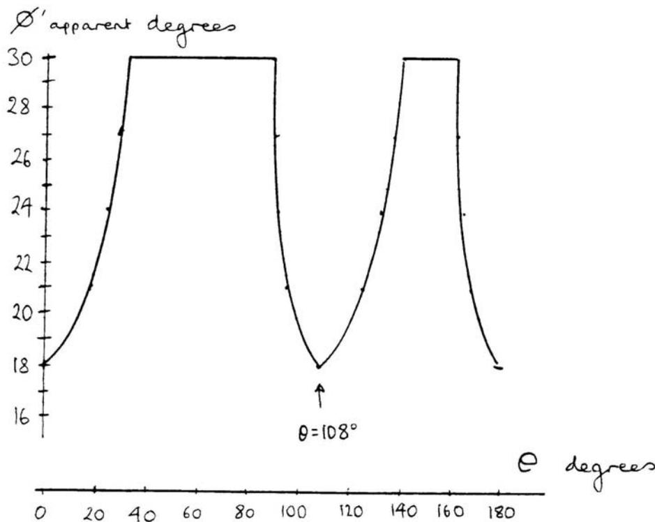
**Figure Q2.8b: apparent effective angle of friction against angle of lamination inclination**
