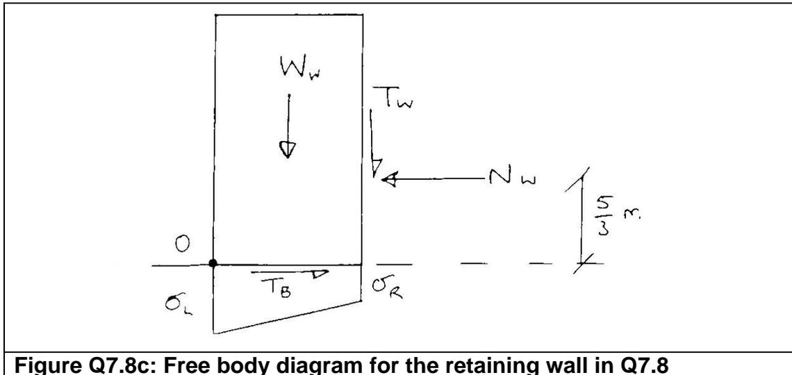
**Figure Q7.8c: Free body diagram for the retaining wall in Q7.8**
