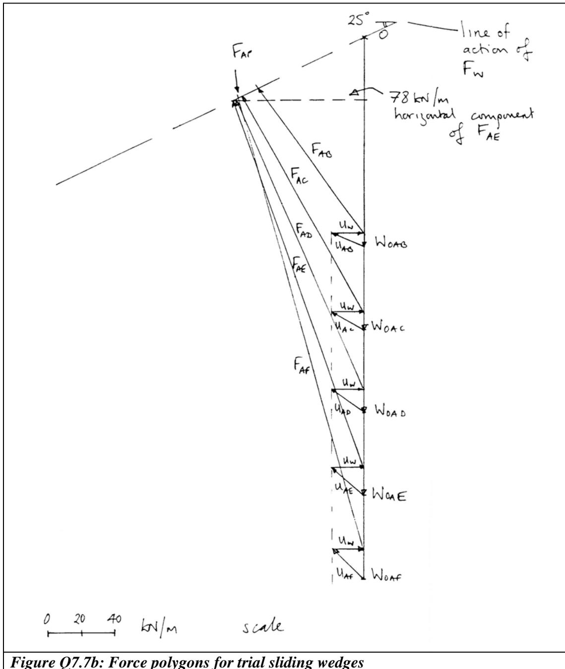
**Figure Q7.7b: Force polygons for trial sliding wedges**
