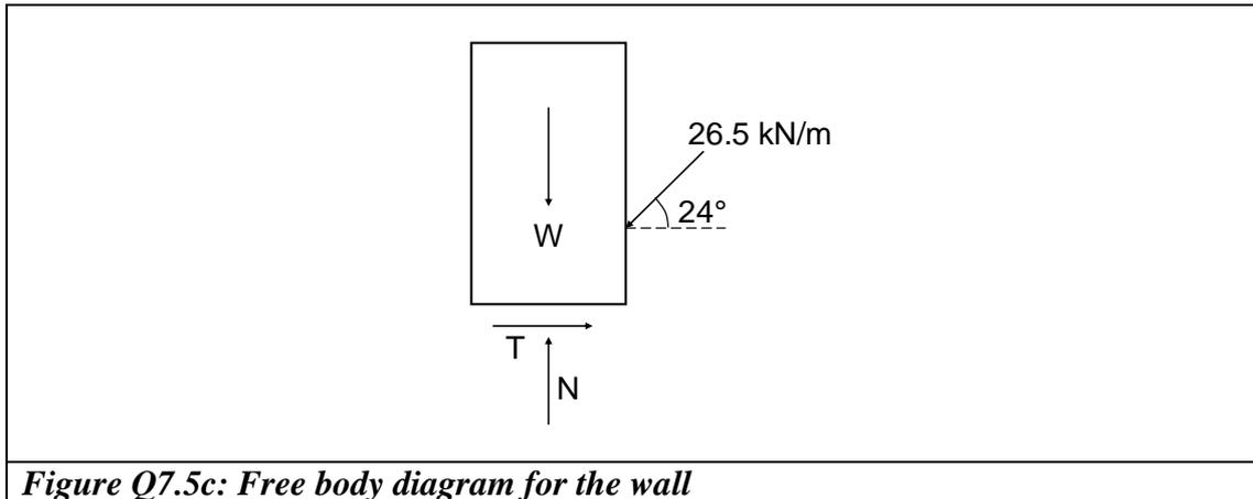
**Figure Q7.5c: Free body diagram for the wall**
