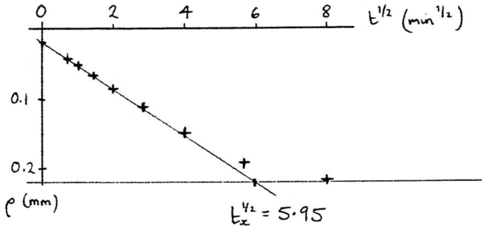
Figure Q4.5: Settlement against  $\sqrt{\text{time}}$
