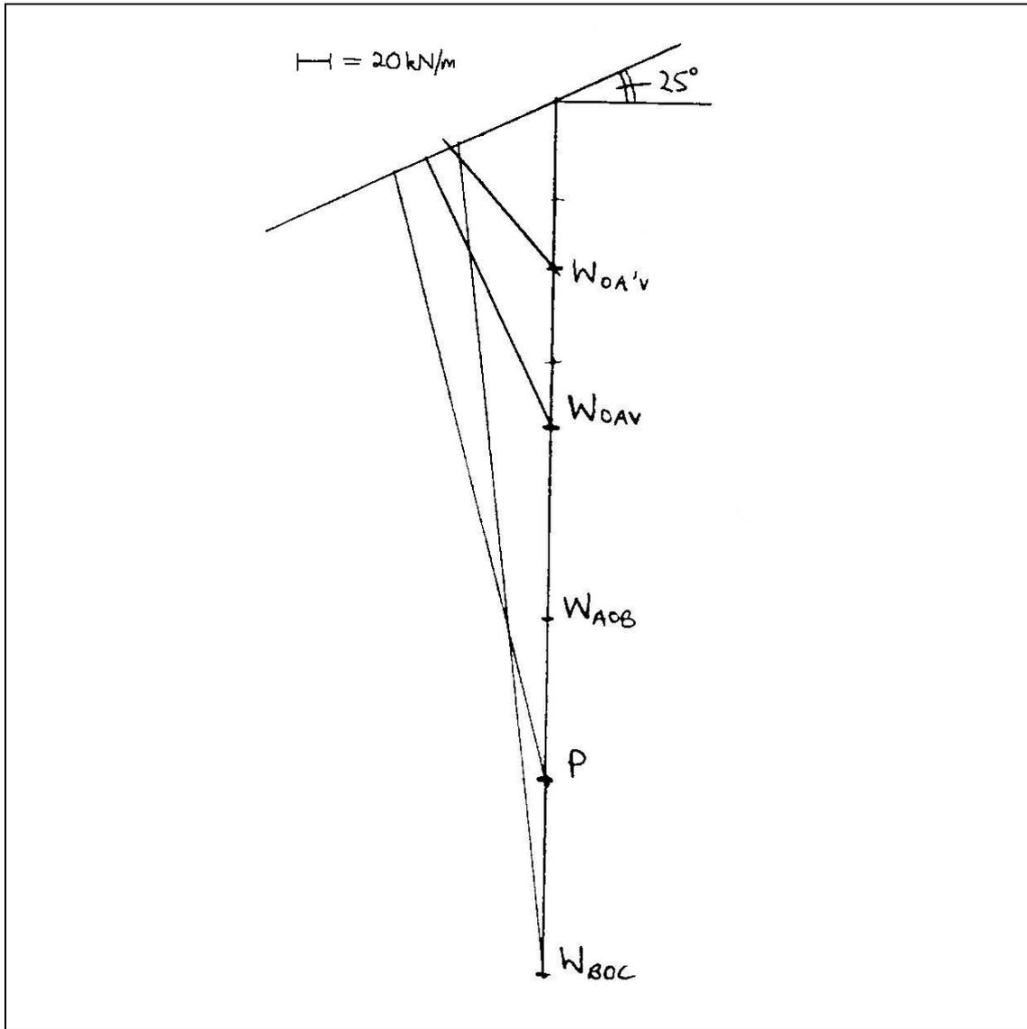
**Figure Q7.6b: Force polygons for trial sliding wedges**
