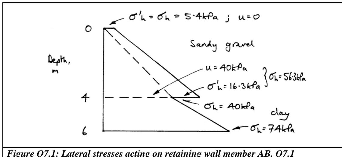
**Figure Q7.1: Lateral stresses acting on retaining wall member AB, Q7.1**
