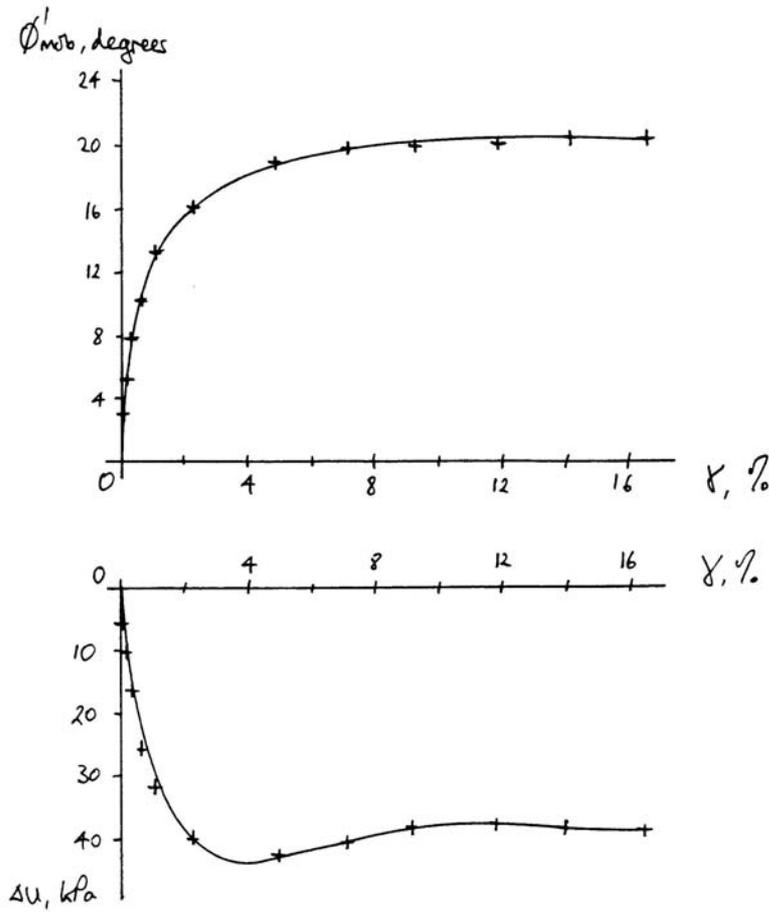
Figure Q5.1a: mobilized strength  $\phi'_{mob}$  and change in pore water pressure  $\Delta u$  against shear strain  $\gamma$
