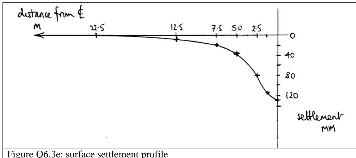
Figure Q6.3e: surface settlement profile
